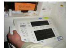
Philips Diagnost Control Panel – Thumb is on the Expose button.
