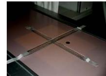
Radio-opaque rulers securely taped to the table. Open collimation boundary is visible.
